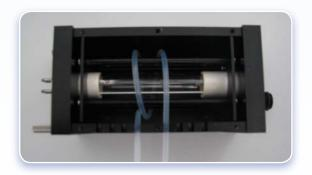
The PN7205 UVD Module runs completely automated and does not need any eluent stirring, which can cause extra artifacts and contamination problems.
