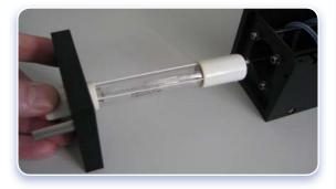
The UVD can be used for flow rates from 0-10 mL/min and is ideal for any aqueous based eluents which show acceptable UV absorption properties. The only spare part is the UV lamp which needs a replacement after a certain operation time (approx. 8000 hours), depending on use and switching cycles. The exact status of the UV light source is displayed via LED at the front cover of the UVD module.
