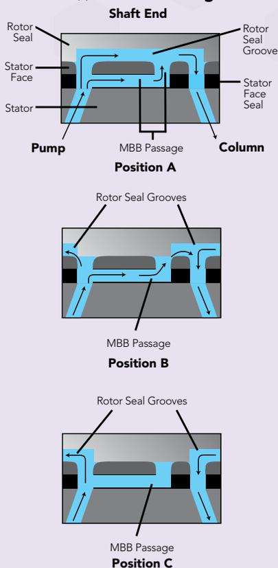
To maintain a constant, desired high-pressure flow, our Make-Before-Break (MBB®) design creates continuous flow between the LOAD and INJECT positions that virtually eliminates pressure transient shock to the system. A passage in the stator face makes a new connection before old connections break. The MBB design — an improvement over bypass-style injectors — does not dilute the sample and is easy to maintain and troubleshoot.
