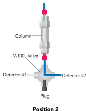
› Your detector switching application may require the flexibility of routing the column effluent to both detectors simultaneously while retaining the ability to isolate each detector. Use our 3-Way Flow Switching Valve ("T"), plugging off the fourth port with the included plug.
