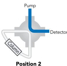
› A typical application for a Right Angle Flow Switching Valve ("L") is column switching, allowing two columns to use one detector. Detector switching is another common application for this valve (see below). Plug off the extra port with the included plug.
