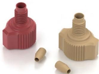
Two-Piece Fingertight Fittings feature a separate ferrule. Use a standard knurled head fitting for traditional fingertight applications, or use a fitting with wings built into the head for extra tightening leverage. A stainless steel hex headed fitting can be used for applications where a wrench may be needed for added tightening torque.
