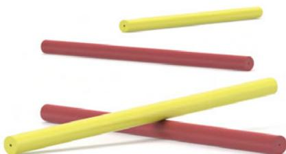
Like the NanoTight™ FEP Sleeves on the previous page, these PEEK Tubing Sleeves are designed to be used with 1/16" OD, 10-32 threaded fittings to adapt capillary tubing to standard coned ports. Made of PEEK polymer, these 1.3" long sleeves can be used up to 125 °C.
