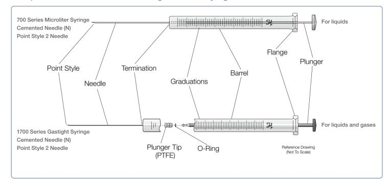
Microliter syringes have a stainless steel plunger which is individually hand-fitted to its matching glass barrel. The hand-fitting process is finely controlled to create a liquid-tight seal between the barrel and the plunger. Plungers for Microliter syringes cannot be interchanged or replaced if damaged.
