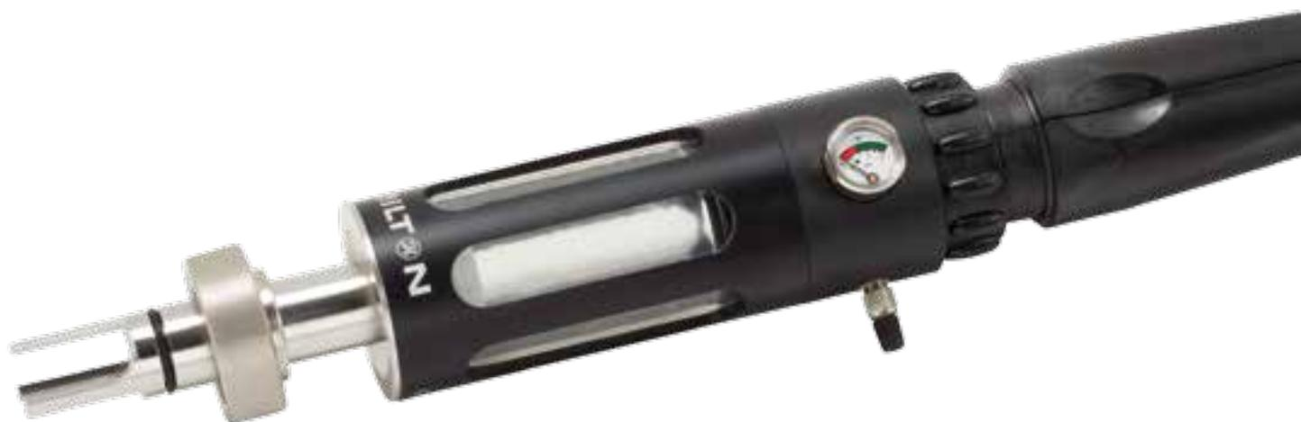
The MasterFit is a housing for pressurizable pH sensors like the ChemoTrode types. The pressurization ensures a constant outflow of electrolyte. This helps to prevent clogging of the diaphragm and poisoning of the electrolyte. The MasterFit can be used in a huge variety of applications mainly in the chemical industry.
