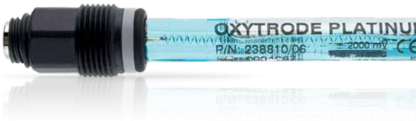
The maintenance free OxyTrode Pt is an ORP sensor designed for processes in the chemical industry and for applications in wastewater treatment. Three high-performance ceramic diaphragms reduce the effect of flow potentials in pipe mounting.
