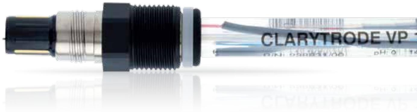
The ClaryTrode sensor is designed for measuring pH in applications containing hydrofluoric acid (HF). HF for example is formed as a by-product of the production of phosphoric acid, which is derived from the mineral apatite. The Everef-L reference cartridge ensures a long lifetime. Because of its two Single Pores liquid junction problems and total break downs are eliminated. The ClaryTrode can be mounted upside down at the bottom of a tank.
