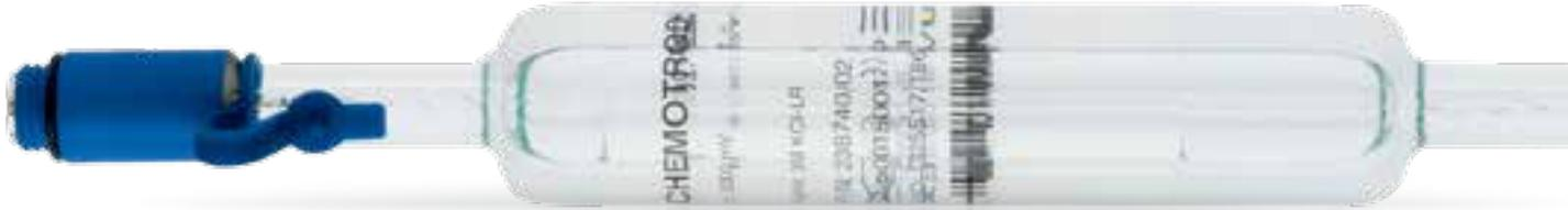
The ChemoTrode ORP is the most robust sensor to measure the oxidation-reduction potential in demanding applications in pharmaceutical and chemical industries. The ChemoTrode has a refill hole which allows refilling the electrolyte and pressurization of the reference electrolyte. Its Everef-F reference cartridge ensures that the reference electrolyte remains free of silver and precipitation of proteins.
