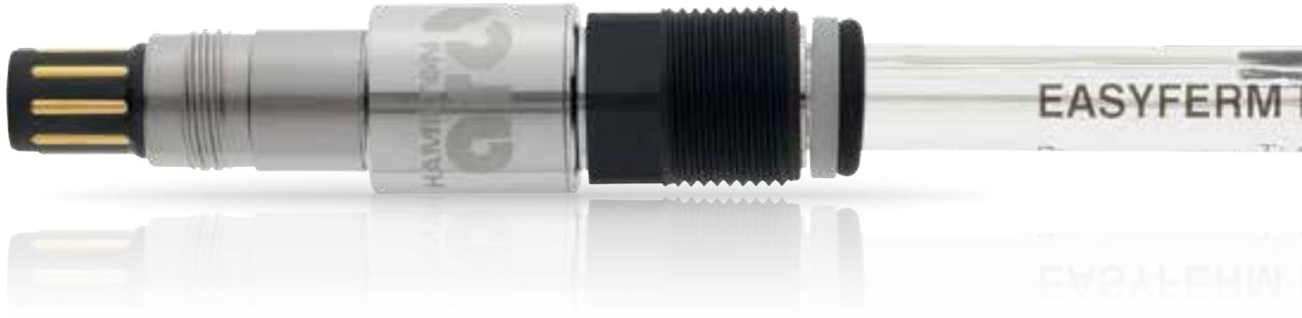
The EasyFerm Plus sensors are designed to withstand demanding applications in pharmaceutical and chemical industries. It is supplied with a pre-pressurized electrolyte which prevents the diffusion of sample into the sensor. The Everef-F reference cartridge ensures that the Phermlyte reference electrolyte remains free of silver and precipitation. It withstands steam sterilization, autoclavation and CIP cleanings.
