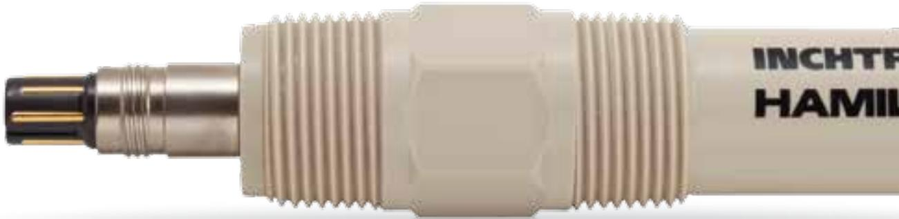
The InchTrode sensors are designed to measure pH in demanding applications in the paper making as well as in the chemical industries. The Single Pore liquid junction guarantees best and fast measuring results because of direct contact between the sample and the Polysolve electrolyte.
