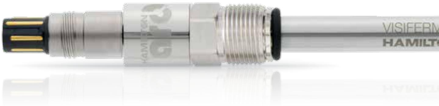
The VisiFerm DO is the first optical oxygen sensor with integrated opto-electronics, having the full functionality of a measuring device with self-diagnostics. It is steam sterilizable, autoclavable and CIP compatible. The VisiFerm requires less maintenance than a classical oxygen sensor as it does not have a mechanically sensitive membrane or a corrosive electrolyte.
