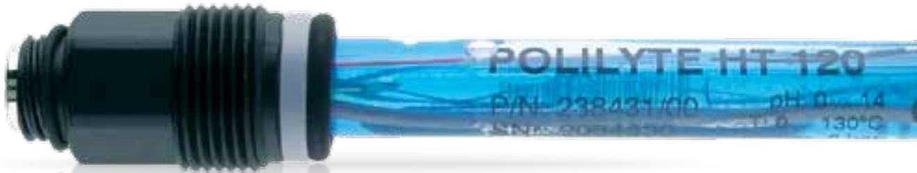
The maintenance free Polilyte HT sensors are designed to withstand demanding applications in chemical and petrochemical industries. The Polilyte HT is the predecessor of the Polilyte Plus.
