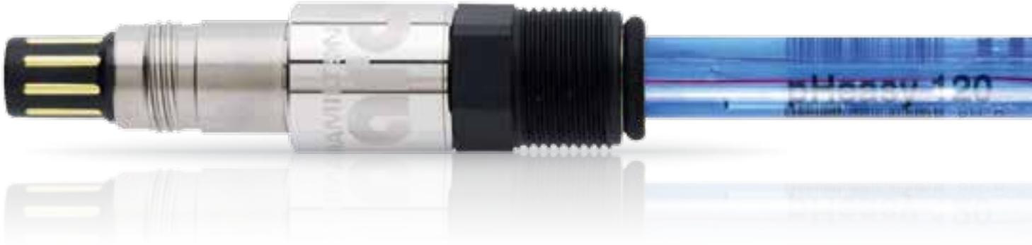
The pHeasy is one of the first pH sensors with a built-in lifetime monitoring without calibration. The second reference electrode helps to detect reference problems and indicates when the sensor has to be changed. It is designed for various applications where monitoring the long-term stability is appreciated like in the chemical industry or in wastewater treatment.
