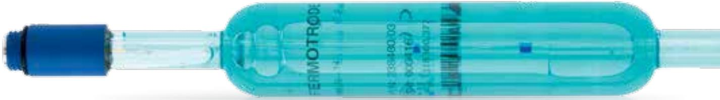
The maintenance free FermoTrode sensors are designed for measuring pH in pharmaceutical and biotechnological industries and fit in the MasterFit and RetractoMaster housings. The Everef-F reference cartridge ensures that the reference electrolyte Skylyte remains free of silver and precipitation. It withstands steam sterilization.
