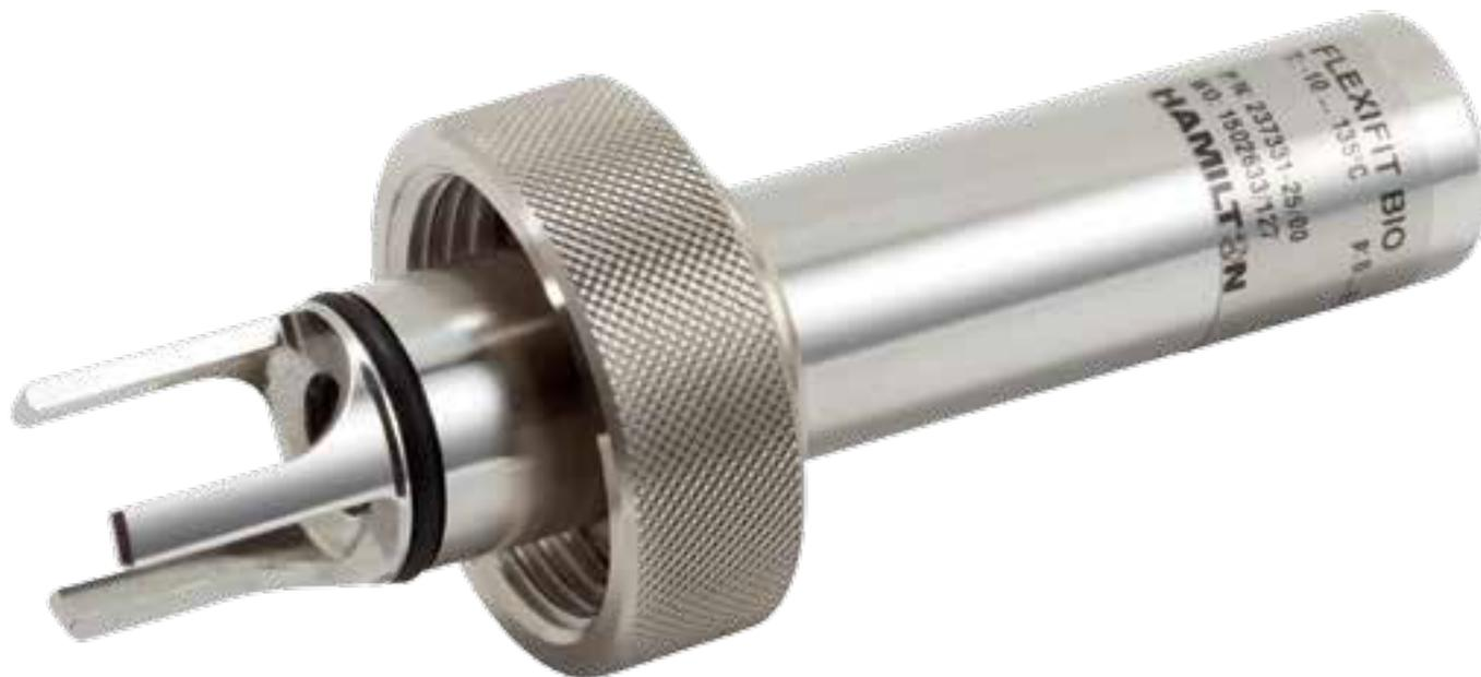
The FlexiFit housings are designed for 120 mm sensors in different kinds of industries. A variety of process connections ensure the usability in the chemical industry as well as in hygienic processes. All FlexiFit have EPDM o-rings and the electropolished surface quality ( $R_a < 0.4 \mu\text{m}$ ) quality is shown on a certificate. They are suitable for autoclavation, CIP and SIP procedures.
