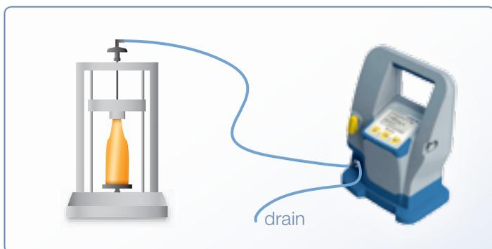
Beverly can be used as shown in the pictures and even beyond. A further application is to check the oxygen content of the exhaust gas of vessels while flushing with CO<sub>2</sub> after cleaning and prior to filling. Measuring the oxygen at this point can help to save time and CO<sub>2</sub>. Even if Beverly stays connected to a pipe or a vessel while CIP is running it's robust stainless steel flow cell prevents damage.
