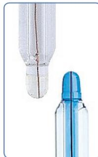
membranes, allowing readings, for example with the FlaTrode™ in small volumes or on flat surface areas. Hamilton “H” glass shows excellent performance and stable measurement values in media with low water content, for example in anhydrous or only partially aqueous solutions. The low alkali error of “H” glass ensures accurate measurements even at high pH values.
