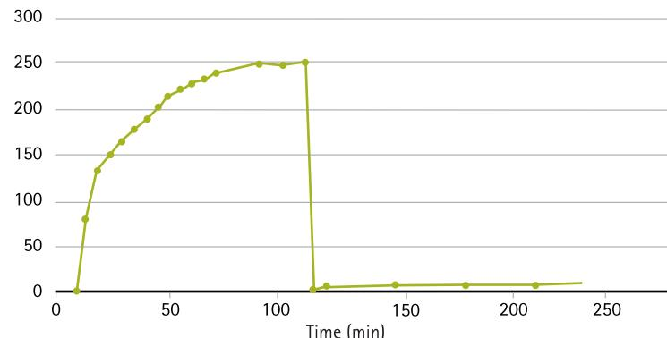
D-Tube™ Dialyzers provide gentle, efficient desalting and excellent protein recovery. A bovine serum albumin (BSA) solution in 2M NaCl was dialyzed against water while water conductivity was monitored. After 100 minutes, conductivity of the water stopped increasing, and it was replaced with fresh water. After 5 hours, 89% of the protein was recovered, and 99.9% of the salt had been removed.
