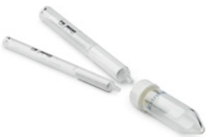
EXtrelut® NT sorbent columns simplify liquid-liquid extraction by replacing separation funnels. Using a single step is more efficient and saves solvent, material and time in contrast to classical funnel separation. With its intuitive working principle, higher recovery and cleaner extraction can be achieved. The aqueous sample is simply applied to the EXtrelut® NT sorbent, which distributes itself as a thin film over the chemically inert matrix and thus acts as a stationary phase.
