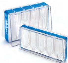
Use the Minicon® static concentrators to concentrate urine and cerebrospinal fluid to intensify proteins that indicate abnormal or pathological states prior to analysis by electrophoresis or immunoelectrophoresis. The B15 unit has 8 cells and can hold up to 5 mL of sample. The CS15 has 10 cells and is suited for volumes up to 2.5 mL. The absorbent pulls solvent and salts through the ultrafilter, concentrating the sample.
