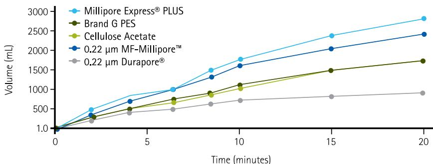
Proven fast flow rate. 47 mm membrane disks with a 0.22 µm pore size were challenged with DMEM with 10% FBS, and the time required to measure each volume was recorded.
