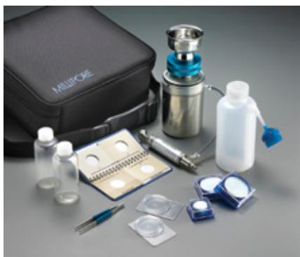
The Patch Test Kit is a complete solution for field-based collection and analysis of hydrocarbon-based hydraulic fluids, bulk chemicals, boiler water, and lubricating oils. It allows the detection of significant changes in cleanliness through dependable, sensitive, colorimetric-based analysis.
