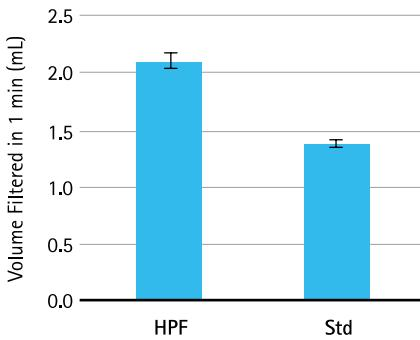
Faster filtration for hard-to-filter solutions. A 25 mm Millex® HPF syringe filter and a standard 25 mm Millex® filter, both with 0.2 µm hydrophilic PTFE membrane, were used to filter a 1% solution of Pepto-Bismol® in Milli-Q® water using a pressure vessel set to 10 psi. Filtrate was collected in tared borosilicate tubes. The Millex® HPF filter enabled filtration of a higher volume of solution in one minute compared to the standard filter.
