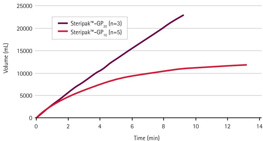
Steripak™ filters deliver fast flow and high throughput. Data show typical flow rates and throughput for 100 cm<sup>2</sup> (Steripak™-GP<sub>10</sub>) and 200 cm<sup>2</sup> (Steripak™-GP<sub>20</sub>) filters using tissue culture medium with 10% serum at 25 psi (1.7 bar).
