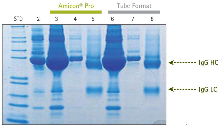
100 µL Protein A beads were mixed with 1 mL rabbit serum (1:10 diluted) and IgG was purified by standard tube protocol or using an Amicon® Pro device. IgG purification was near complete using either method.
