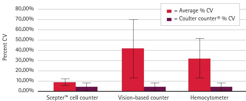
The average percent coefficient of variation (CV) for each counting method shown was calculated using cell concentration measurements at 50,000 cells/mL samples of 19 different cell lines. The Scepter™ cell counter is more precise than vision-based counting and hemocytometry, and approaches the precision of the Coulter Counter® standard (maroon bars). Error bars represent standard deviation.
