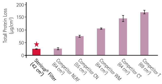
13 mm disks were cut out from different filtration devices (n=3). Protein binding was quantified by incubating discs in 1 mL tracer (1 mg/mL goat IgG in PBS containing <sup>125</sup>I-goat IgG at 0.1 µCi/mL). After 2 h of shaking at RT, the tracer solution was aspirated. Disks were washed 3X in PBS then assayed for bound radioactivity.
