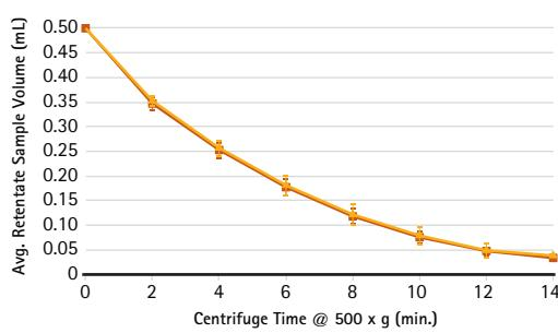
Figure 1. Equally fast ultrafiltration flow of Microcon® DNA Fast Flow (Orange) and Microcon® DNA Fast Flow PCR Grade (Yellow) devices as determined by measuring retentate volume at various time intervals and plotting retentate volume vs. centrifugation time. Each point represents the mean and standard deviation of four replicates.
