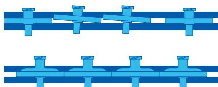
The domed housing of automation-compatible 25 mm Millex® syringe filters enables smooth, reliable delivery by eliminating shingling between filters in the transport rack.
