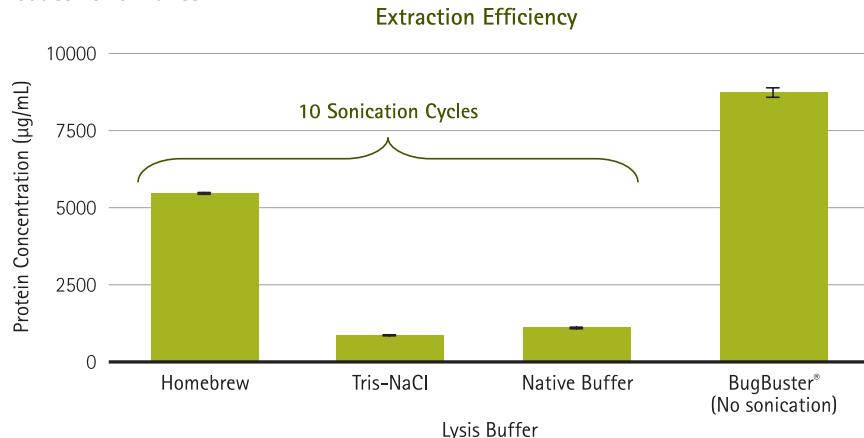
Higher extraction efficiency of BugBuster® reagent (with added Benzonase® nuclease and rLysozyme™ solution), even without sonication, compared to three other lysis buffers that were used with 10 cycles of sonication. Cleared cell lysates were spotted on assay cards and quantified using the Direct Detect® spectrometer. Bars represent mean and standard deviation (n=3).
