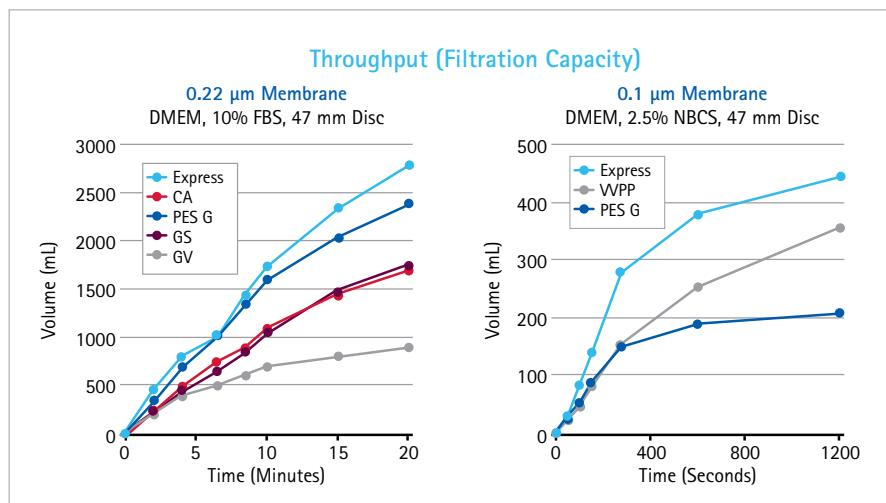
Figure 3. Several membrane types were compared for throughput or filtration capacity. 47 mm discs were challenged with either DMEM, 10% FBS (0.22 µm filters, left), or with DMEM, 2.5% NBCS (0.1 µm filters, right). In both cases, the Millipore Express® (PES) filters exhibited the highest filtration capacity.
