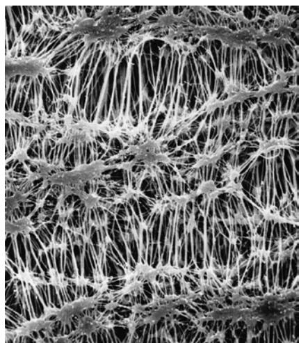
Fluoropore™ Membrane is a hydrophobic, polytetrafluoroethylene (PTFE) polymer membrane bonded to a high density polyethylene support. (Catalogue numbers containing "FHUP" have no backing.) Fluoropore™ Membranes provide broad chemical compatibility, high flow rates and consistency.
