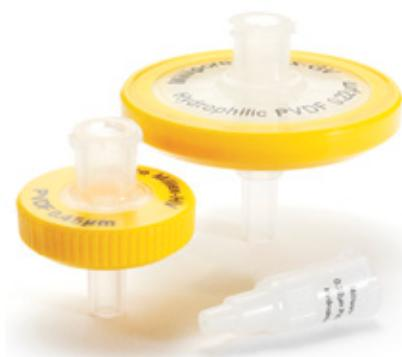
Non-sterile Millex® syringe filters with hydrophilic Durapore® (PVDF) membrane provide high flow rates and throughput, low levels of extractables and broad chemical compatibility. Hydrophilic PVDF membranes bind far less protein than nylon, nitrocellulose membranes, or PTFE membranes. Syringe filters are available in two pore sizes and three diameters to optimize results.
