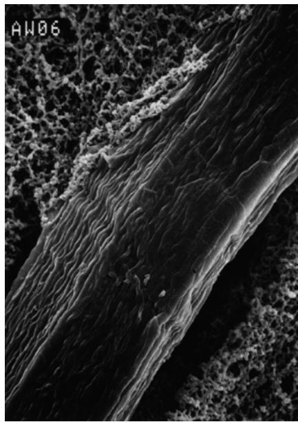
Reinforced prefilter membranes can be used to remove contaminants from a variety of liquids and gases. The filters have a high dirt-holding capacity and a low pressure drop, which makes them ideally suited for reducing contaminant levels in advance of sterilizing-grade filters. Reinforced prefilter membranes are made from non-shedding materials. The filters retain contaminants on the surface of the cellulose membrane.
