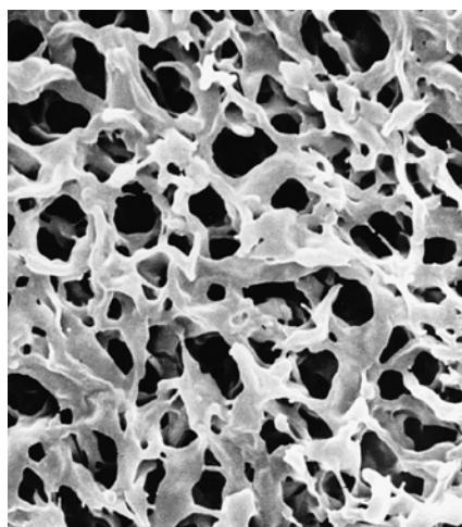
Lowest protein binding with Durapore® PVDF membrane. Membrane disks with a 0.22  $\mu\text{m}$  pore size were exposed to a 1 mg/mL solution of  $^{125}\text{I}$ -labeled IgG. The chart shows protein binding after incubation (normalized to membrane surface area).
