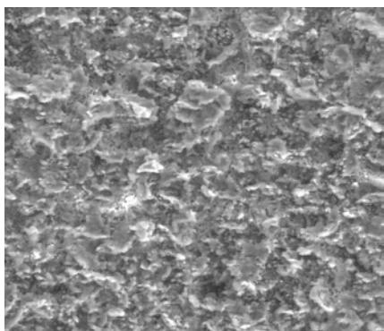
Mitex™ PTFE Membrane is unaffected by almost all liquids, including organic solvents, concentrated acids and bases, propellants, and cryogenic fluids. Mitex™ membrane is unbacked, yet is easy to handle, combining the convenience of a backed membrane with the versatility of a pure PTFE membrane.
