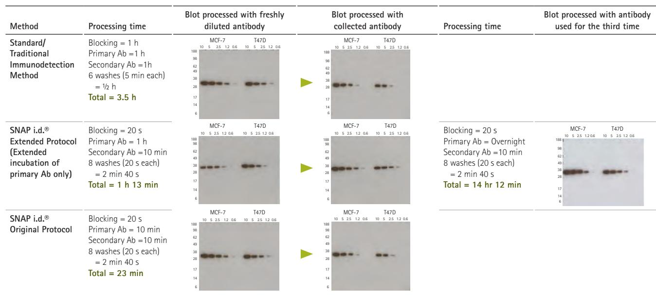
Figure 2. Two-fold dilution series of breast cancer cell lysates (MCF-7 and T47D, 10 to 0.6 µg total protein) were subjected to SDS-PAGE and transferred to blotting membranes in seven identical blots using three different immunodetection protocols as described above. The seven blots were probed with anti-PP2A, which was either freshly diluted, collected or recovered for a second time.
