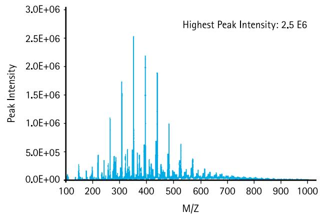
Millex® filters feature low extractables. Mass spectrometry detects few extractable impurities from Millex® syringe filters containing 0.45 µm pore hydrophilic PTFE membrane (A). In contrast, a syringe filter containing 0.45 µm pore polypropylene membrane from another vendor (B) shows significant leaching of impurities.
