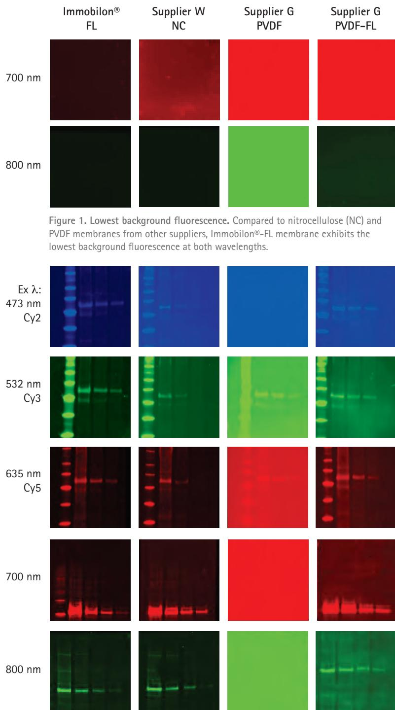
Figure 1. Lowest background fluorescence. Compared to nitrocellulose (NC) and PVDF membranes from other suppliers, Immobilon®-FL membrane exhibits the lowest background fluorescence at both wavelengths.
