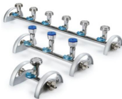
The EZ-Fit® Manifold is designed to increase laboratory workflow efficiency and make laboratory filtration easier. It features quick-fit connections for assembly and disassembly without tools and a low profile to increase operator comfort. Plus, all internal areas are accessible for easy cleaning, facilitating biofilm prevention. Different filtration heads, all with quick-fit connections, make the manifold
