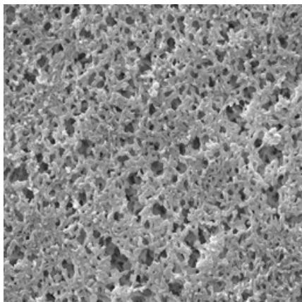
Nylon filters are compatible with a broad range of solvents. Two types are available: membrane filters with pore sizes ranging from 0.20 to 1.2 µm and woven net filters with mesh openings ranging from 10 to 180 µm.
