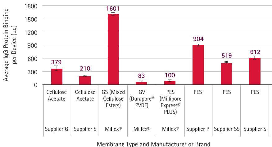
Millex® filters with PVDF and PES membranes exhibit significantly less protein binding than other syringe filters. Membrane disks cut from various syringe filters were offered a 1 mg/mL tracer solution (1 mg/mL goat IgG in PBS with 0.1 µCi/mL of <sup>125</sup>I-goat IgG). The chart shows the amount of protein bound after two hours of shaking and three washes with PBS.
