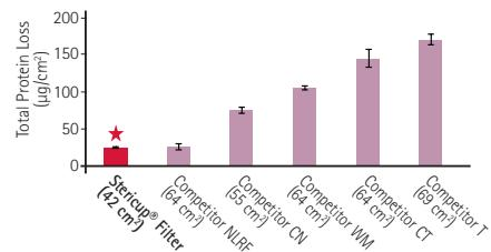
13 mm disks from were cut out from different filtration devices (n=3). Protein binding was quantified by incubating discs in 1 mL tracer (1 mg/mL goat IgG in PBS containing  $^{125}\text{I}$ -goat IgG at 0.1  $\mu\text{Ci}/\text{mL}$ ). After 2 h of shaking at RT, the tracer solution was aspirated. Disks were washed 3X in PBS then assayed for bound radioactivity.
