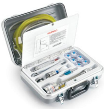
The Fluid Sampling Kit is a complete solution for field-based fluid collection and contamination analysis. The stainless steel sampler assembly plugs into a quick-release valve installed in the system line, which allows a measured quantity of liquid to pass through the monitor. A valved syringe serves as a pump to remove residual liquid from the monitor. Kit is compatible with our 37 mm contamination monitors and matched-weight monitors.
