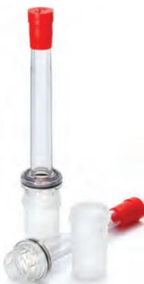
The Centrifree® Ultrafiltration device with Ultracel® regenerated cellulose membrane is ideal for separating free from bound microsolutes in serum, plasma, and other biological samples. The device is licensed for research use and *in vitro* diagnostic use. The device holds a sample volume of 1 mL with a hold-up volume of 10 µL.
