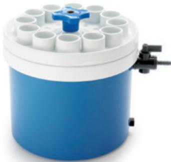
Simultaneously vacuum filter 12 samples for rapid analysis of retentate or filtrate. Numbered positions on the filter plate assure accurate sample tracking. Sealing stoppers maintain vacuum on unused sample cups. Accessory extension barrels increase sample volumes from 15 to 50 mL.
