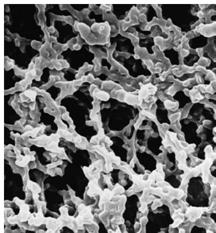
Biologically inert mixtures of cellulose acetate and cellulose nitrate have made MF-Millipore™ membrane filters one of the most widely used membranes in analytical and research applications.
