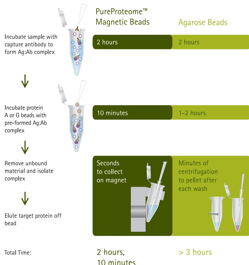
High speed immunoprecipitation with magnetic beads compared to agarose. In parallel indirect immunoprecipitations, PureProteome™ magnetic beads offered a 50% reduction in incubation time while yielding results equivalent to agarose beads.
