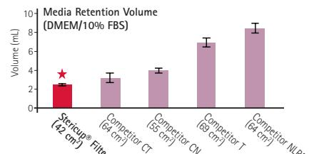
500 mL of DMEM+10%FBS was filtered to completion through various 0.22  $\mu\text{m}$  hydrophilic PES membrane filtration devices. Filtration rates and retention volumes were calculated (n=3).
