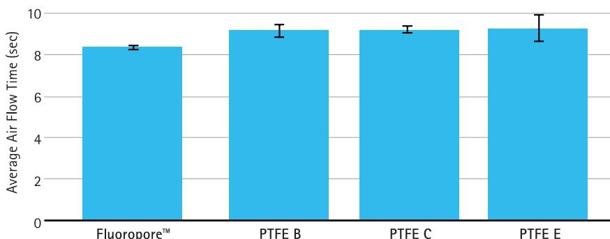
Faster flow and less variability than competitors for consistently strong performance. Air flow through PTFE membranes from various suppliers was measured using a Gurley 4110 Densometer with 0.1 in<sup>2</sup> aperture size and 100 cc air setting and a 20 oz cylinder.
