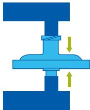
A rigid domed housing design helps prevent backpressure, which can cause a workstation shut-down.
