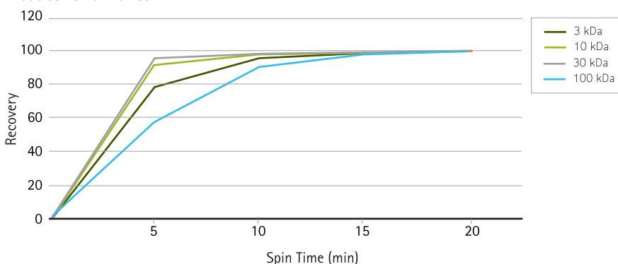
Amicon® Ultra 4 mL filters provide fast spin times with excellent recovery. Solutions of four different proteins (3 kDa cytochrome C, 10 kDa cytochrome C, 30 kDa BSA and 100 kDa IgG) were concentrated using Amicon® Ultra 4 mL filters. Average percent recovery and spin times were recorded. Data show that more than 95% of all protein was recovered in 15 minutes or less.
