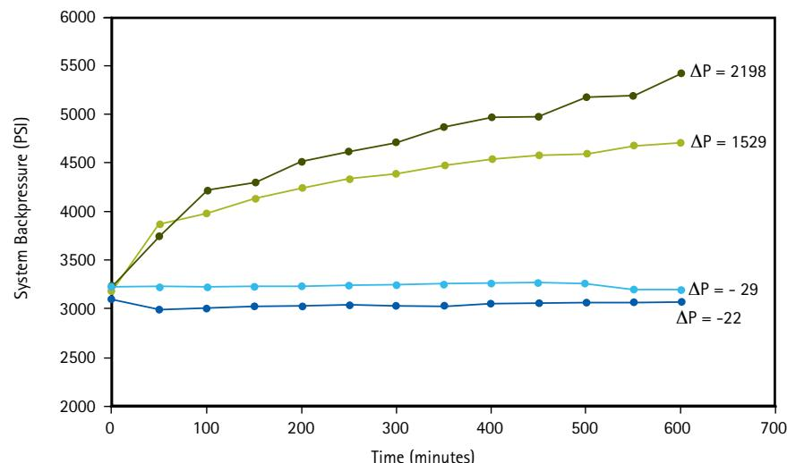
Figure 1. Filtration through 0.2  $\mu\text{m}$  hydrophilic PTFE Millex® filters prevents backpressure buildup on a UHPLC system. Water and acetonitrile were passed through polypropylene or PTFE syringe filters (as indicated in legend), then used 1:1 (v/v) to prepare the mobile phase for UHPLC. The system was run at 0.25 mL/min for 600 min with backpressure recorded every 50 min.  $\Delta\text{P}$  represents total change in backpressure after 600 min.
