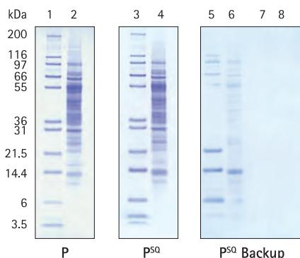
Immobilon®-PSQ membrane prevents the proteins from blowing through the membrane, increasing protein signal. Molecular weight standards (lanes 1 and 3) and calf liver lysate (lanes 2 and 4) were transferred to Immobilon®-P or Immobilon®-PSQ membranes. A sheet of Immobilon®-PSQ membrane was placed behind the primary membranes to capture proteins that passed through (lanes 5 and 6 behind Immobilon®-P membrane; lanes 7 and 8 behind Immobilon®-PSQ membrane).
