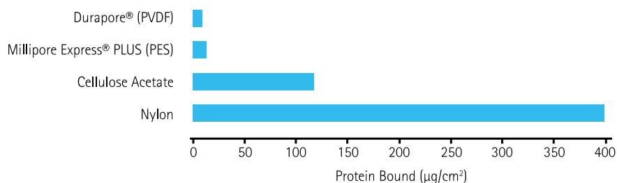
Lowest protein binding with Durapore® PVDF membrane. Membrane disks with a 0.22 µm pore size were exposed to a 1 mg/mL solution of <sup>125</sup>I-labeled IgG. The chart shows protein binding after incubation (normalized to membrane surface area).
