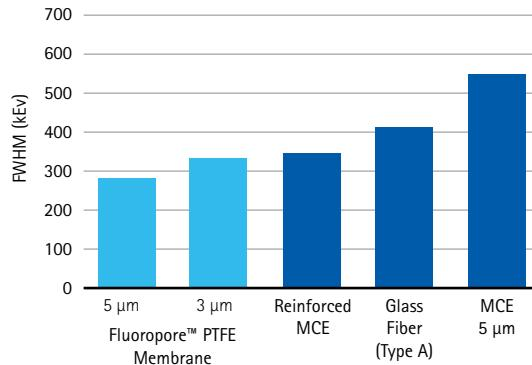
Lower pressure drop, lower FWHM\* measurements. Merck Millipore's Fluoropore™ PTFE membranes exhibit lower pressure drop (A) and collect particles on the surface , providing better detection efficiencies and lower FWHM measurements (B). Room air was collected at 1.7 m<sup>3</sup>/h (1 standard cubic foot/min).
