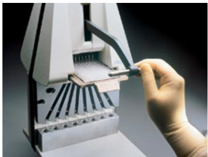
MultiScreen® column loaders let you combine the cost savings of bulk media with the convenience of 96-well filtration plates. All 96 wells are loaded simultaneously and uniformly, eliminating the need for pipetting slurries or using prepacked columns.
