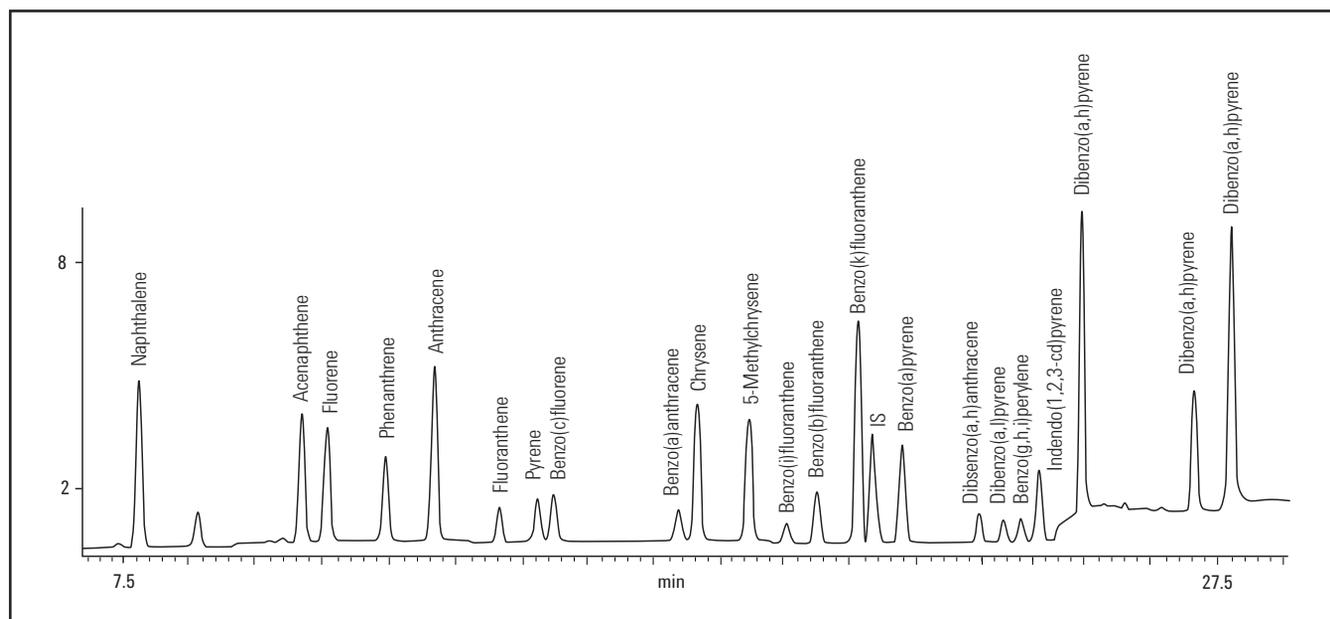
HPLC/FLD chromatogram of a 5  $\mu$ L injection of the 20 ppt PAH standard solution on the Agilent Pursuit 3 PAH column
