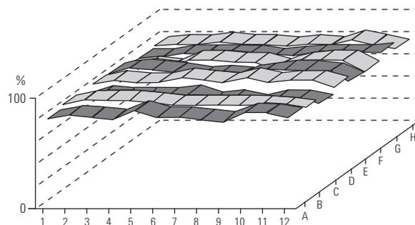
Note the high recovery (y axis) with an average deviation across the 96 wells of just 3.2% (well positions are shown on the x and z axes). SPEC provides the predictable flow characteristics analysts require for true walk-away automated processing. With SPEC you need not worry about clogging, and as an added benefit, the typically low vacuum pressure requirement prevents cross-talk (e.g. spraying of fast running eluates between wells in the collection plate).
