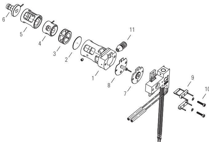
5975/5973 MSD Chemical Ionization (CI) ion source assembly
