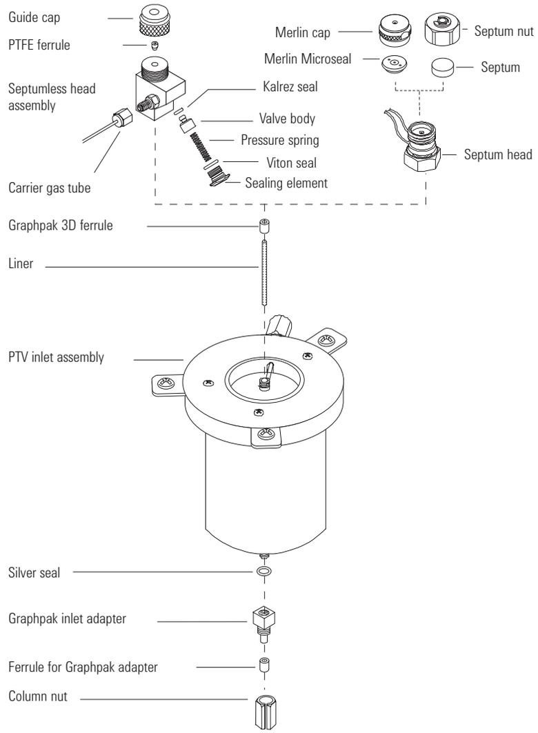
Programmable Temperature Vaporizing (PTV) Inlet assembly
