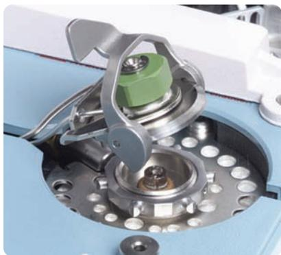
Available exclusively from Agilent, the Flip Top has a levered arm that attaches to any 6890/6850/5890 insert weldment and locks to the injection port using an adapter ring screwed onto the inlet. Once installed, the user simply lifts the arm of the Flip Top which releases the insert weldment from the injection port, and allows instant access to the liner. The process is simply reversed to reseal the weldment to the port.
