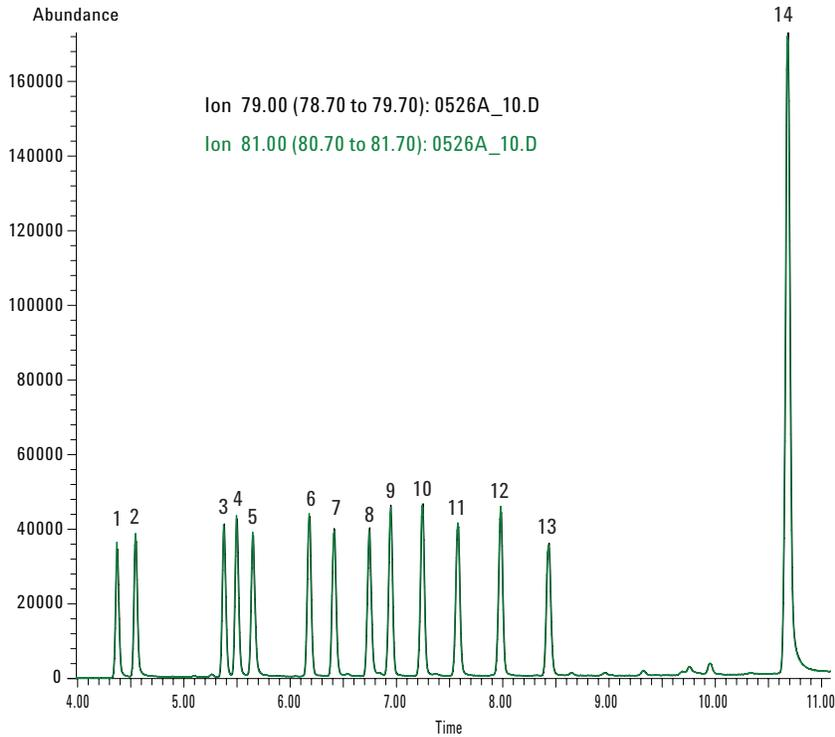
**Figure 1.** GC-ICP-MS chromatogram of 10 ppb PBDE standard mix.
