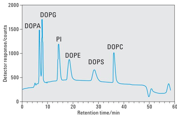
**Figure 1.** Separation of six chemically defined phospholipids in standard mixture on YMC Pack Diol-120 column (250 x 4.6 mm, 5  $\mu$ m) with ICP-MS detection of phosphorus at  $m/z$  ratio 31 (5  $\mu$ L injected, 0.6 mL/min, each peak corresponds to ~15 ng of phosphorus).
