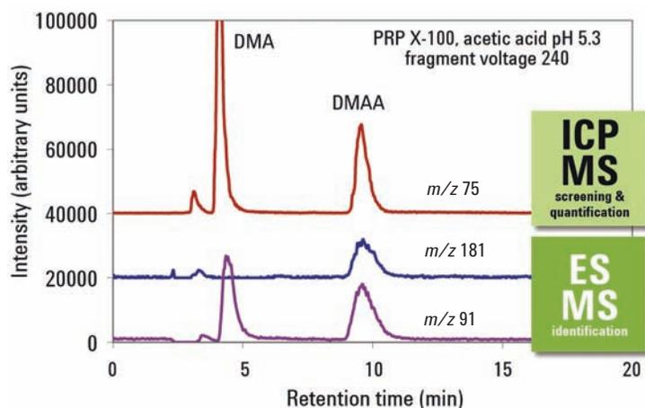
**Figure 1.** First identification of dimethylarsinoyl acetate (DMAA) using HPLC-ICP-MS/ES-MS. The main metabolite dimethylarsinic acid (DMA) is also shown.
