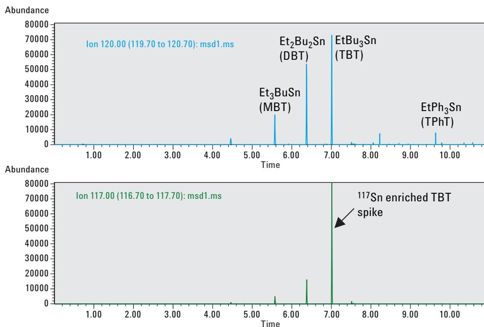
**Figure 1.** GC-ICP-MS chromatogram of a sediment extract after ethylation.
