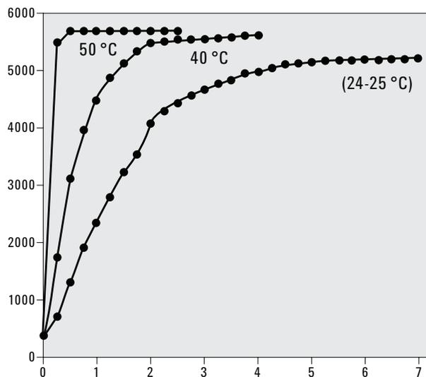
Figure 2. Rate of formation of stable Cr(III)-EDTA complex as a function of time and temperature.
