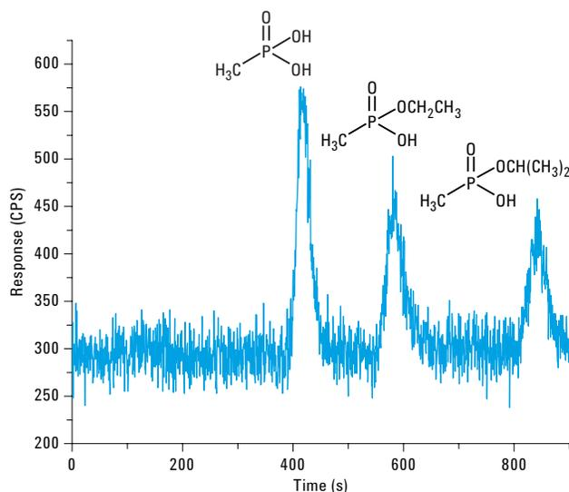
**Figure 1.** Separation of MPA, EMPA, and IMPA in a standard mixture.
