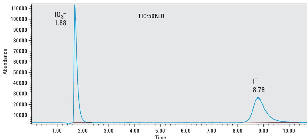
**Figure 1.** IC-ICP-MS chromatogram of 50 nmol/L iodate and iodide standard solution (0.01% KOH medium, mobile: 0.03 mol/L ammonium carbonate).
