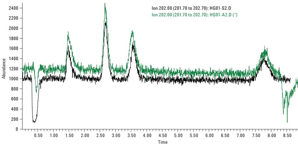
**Figure 2.** Overlaid HPLC-ICP-MS ion chromatograms of 100 ng/L Hg species standards in pure water (upper) and in 3% NaCl (w/v, lower) (20 µL loop).
