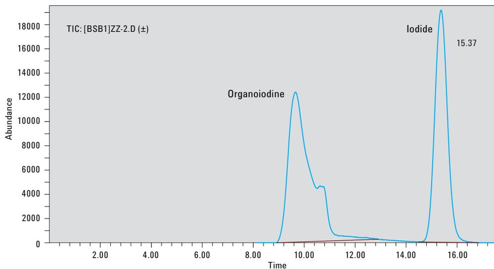
**Figure 2.** SEC-ICP-MS chromatogram of organoiodine and iodide from a groundwater sample.
