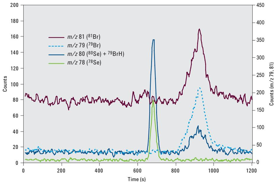
**Figure 1.** Chromatogram of natural water "C" showing interference from bromine hydride elutes after the selenate peak.
