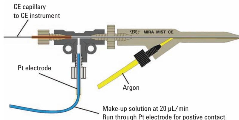
**Figure 1.** Cutaway view of Burgener MiraMist CE interface.
