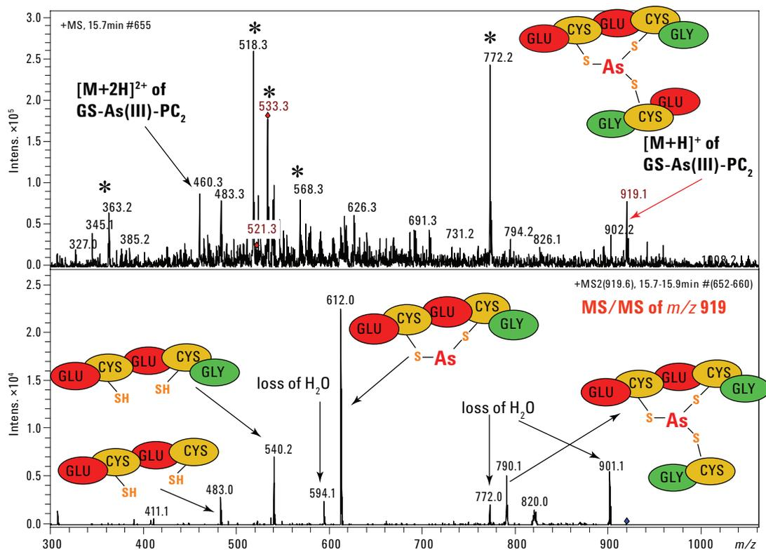
Figure 2. ESI mass spectrum and MS/MS results from the  $M-H^+$  signal of GS-As(III)-PC<sub>2</sub>.
