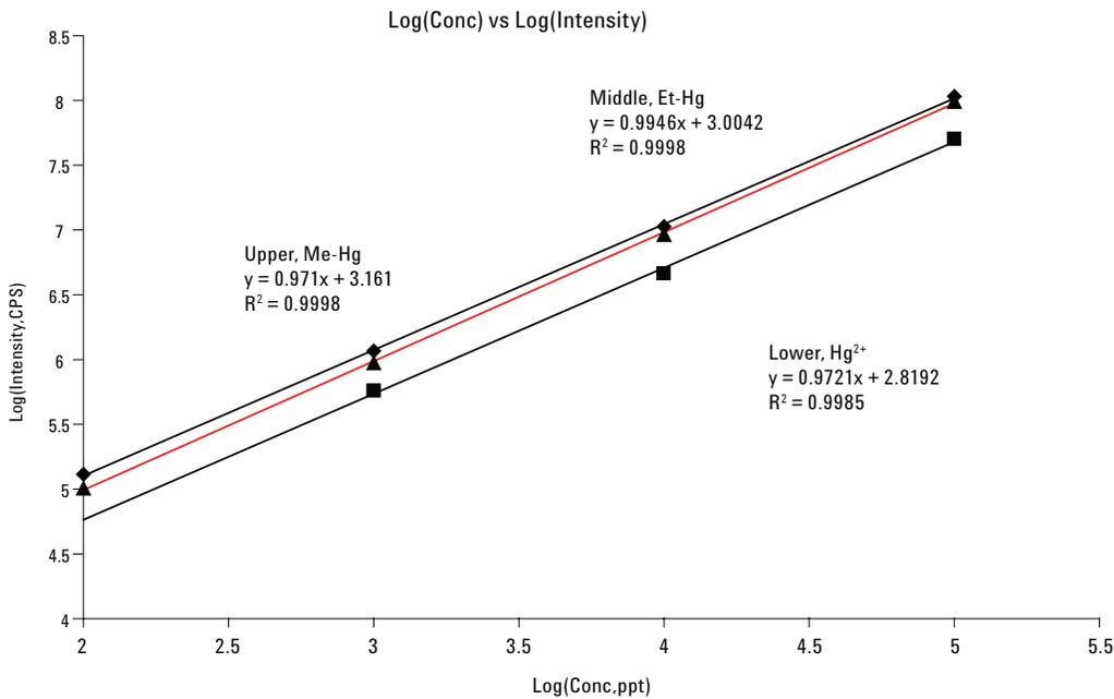
**Figure 1.** Calibration curves for MeHg, Hg<sup>2+</sup> and EtHg.
