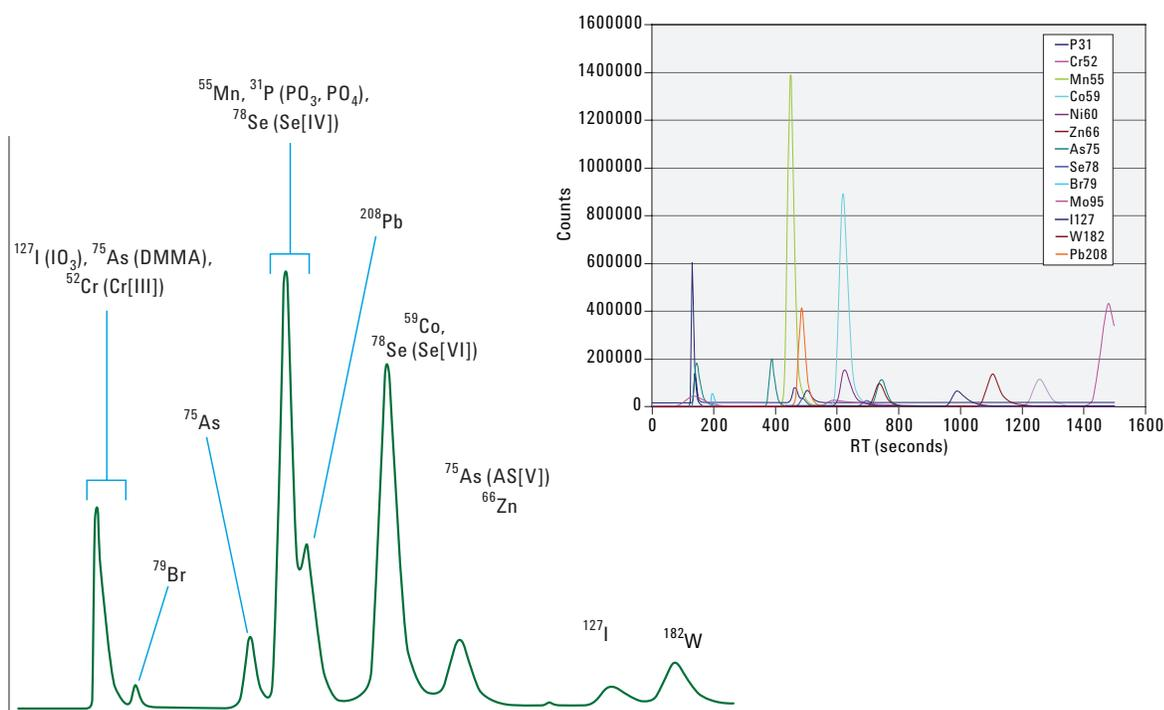
**Figure 3.** Total ion chromatogram depicting simultaneous speciation of multiple elements. Inset shows extracted ion chromatograms of the 13 elements measured. Because of the elemental specificity of ICP-MS, it is not always necessary for each species to be chromatographically resolved.
