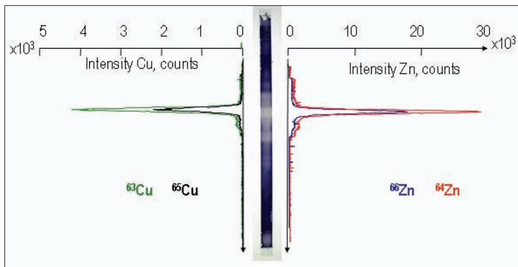
**Figure 1.** Imaging of Cu and Zn in SOD separated by IEF and analyzed by LA-ICP-MS.
