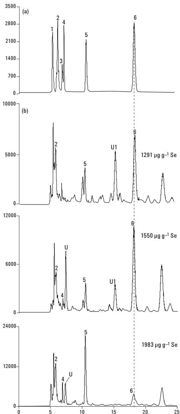
**Figure 1.** RP HPLC-ICP-MS chromatograms of (a) a Se standard mixture containing 3  $\mu\text{g/L}$  Se as Se(Cys)2 (peak 1), 2.5  $\mu\text{g/L}$  Se as selenite (peak 2), 5  $\mu\text{g/L}$  Se as SeMC (peaks 3 and 4) and SeMet (peak 5), and 25  $\mu\text{g/L}$  Se as  $\gamma$ -glutamyl-SeMC (peak 6) and (b) the 1:5 diluted Se-yeast water extracts.
