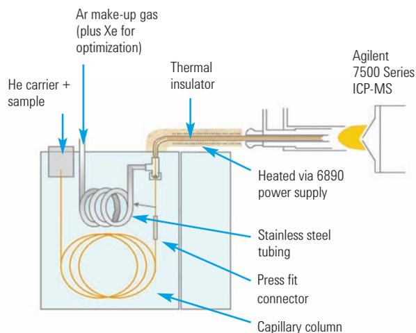
**Figure 1.** Schematic diagram of Agilent GC-ICP-MS system.
