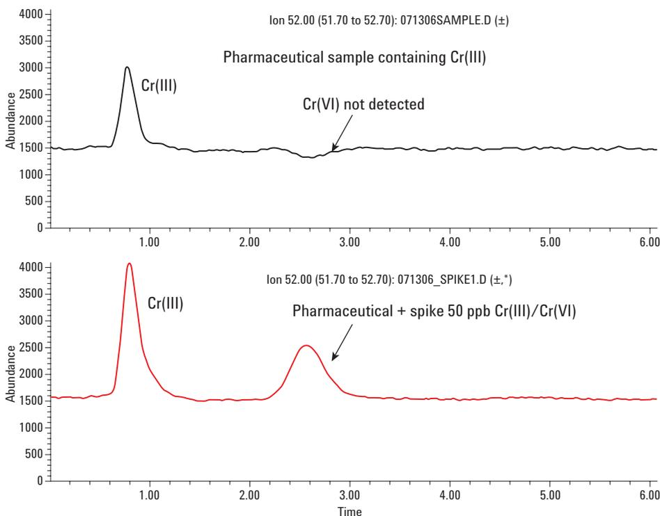
**Figure 1.** Chromatograms showing separation and identification of Cr(III) and Cr(VI).
