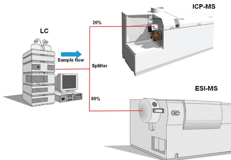
**Figure 1.** Schematic showing a typical LC-multi-MS arrangement.
