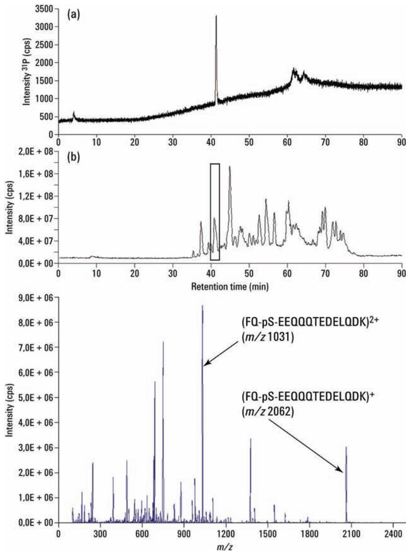
**Figure 1.** (a)  $^{31}\text{P}$  and ESI-TIC peaks of beta-casein in separated by Cap-LC at  $4\ \mu\text{L}\ \text{min}^{-1}$  flow rate. (b) Data deconvolution of the ESI-TIC peak corresponding to the  $^{31}\text{P}$  peak in Figure 1a. Reprinted with permission of ABC.
