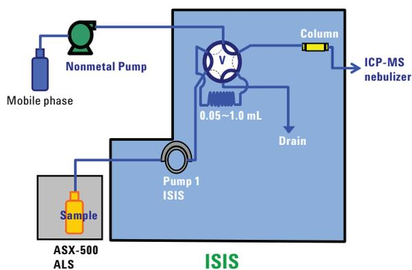
Figure 1. Schematic of the IC-ICP-MS arrangement.
