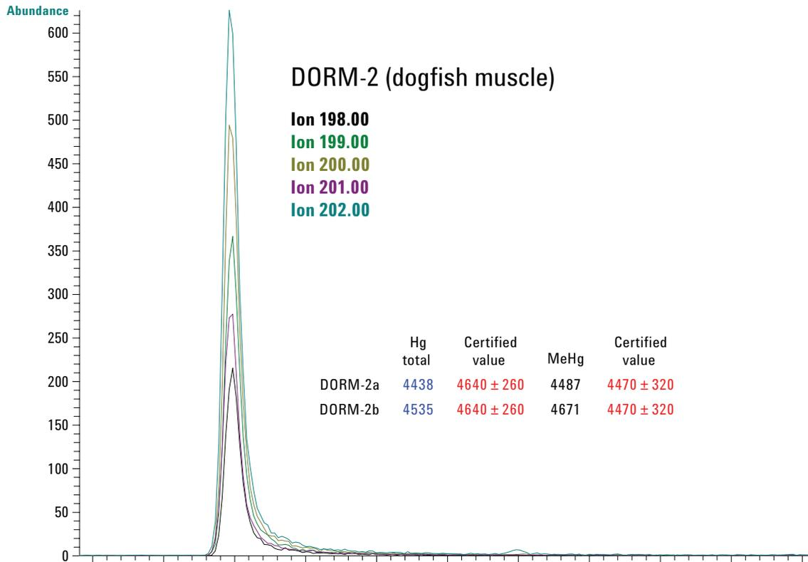
**Figure 1.** Extracted ion chromatograms (overlaid) for mercury in DORM-2 dogfish muscle.
