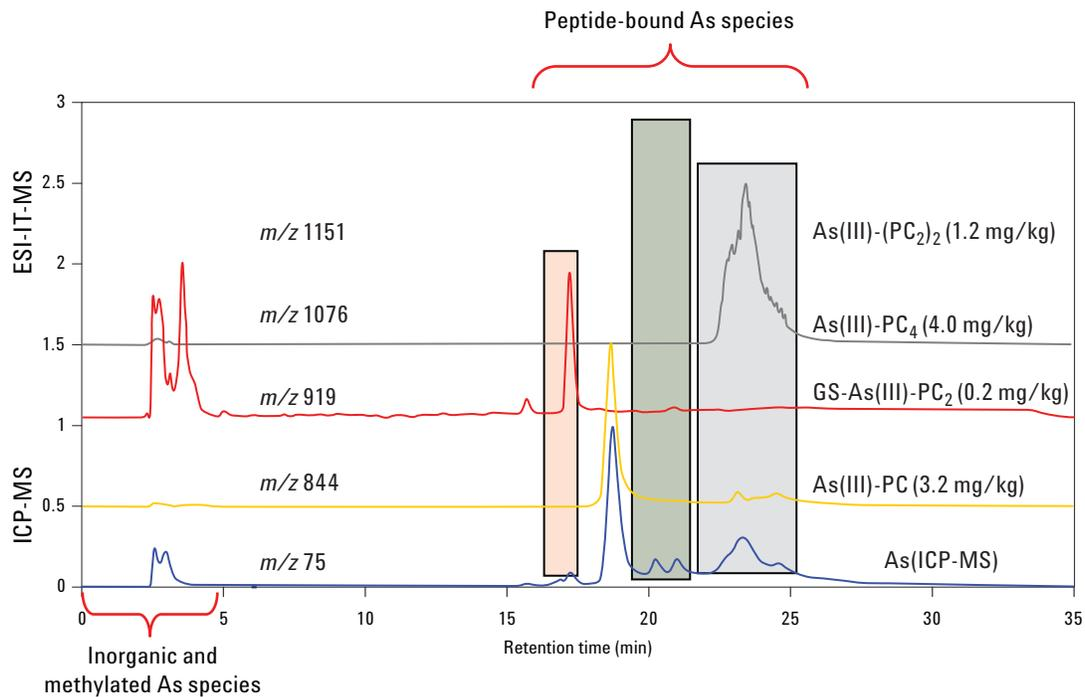
Figure 1. Overlaid ion chromatograms of from electrospray MS and ICP-MS showing phytochelatin arsenic complexes.
