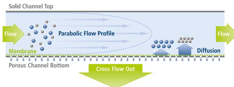
Figure 1: Schematic of the AF4 separation principle.
