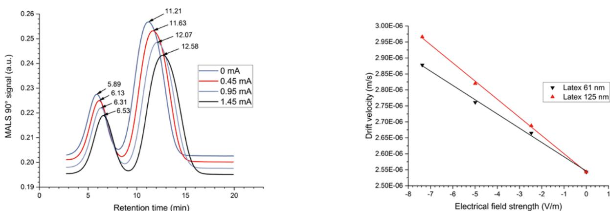
Figure 3: EAF4-MALS fractograms of the investigated nanoplastics particle mixture obtained for four different electrical field strengths (left). Differential velocity versus electrical field strength plot to determine the electrophoretic mobility of the two nanoplastic particles in the mixture (right).
