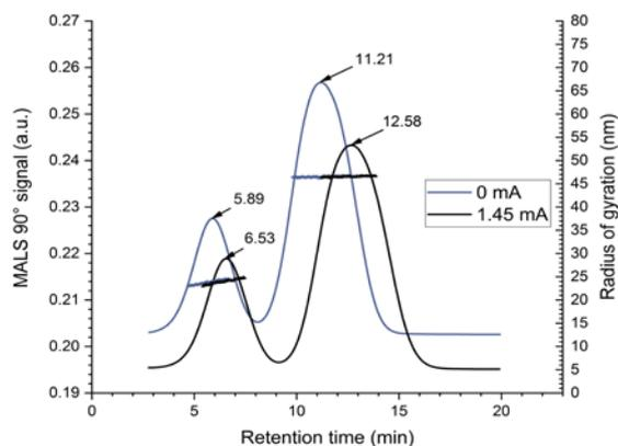
Figure 2. EAF4-MALS fractograms of the investigated nanoplastics particle mixture with and without application of an electrical field (black and blue graph, respectively). The blue and black dotted lines display the radii of gyration obtained from MALS indicating no influence of the electrical field on the particle size.
