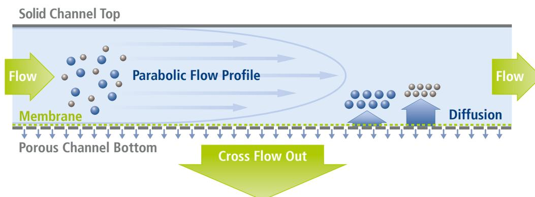
Figure 1: Schematic of AF4 principle.
