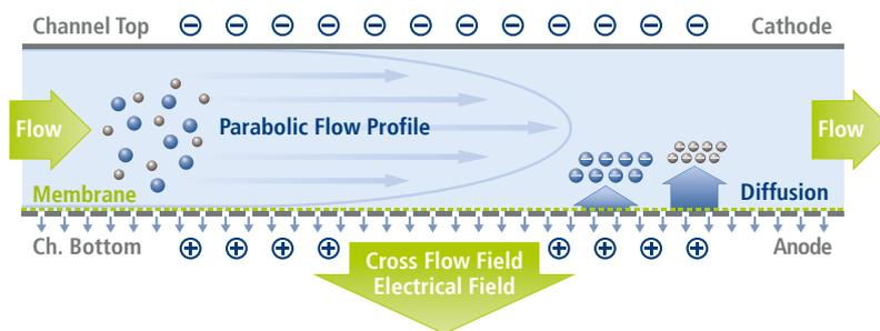
Figure 2: Schematic of the fractionation in an EAF4 channel both by size and surface charge.
