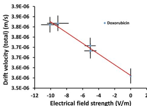
Figure 4: Drift velocity vs. electrical field strength plot to determine the electrophoretic mobility of the Liposomal Doxorubicin sample.
